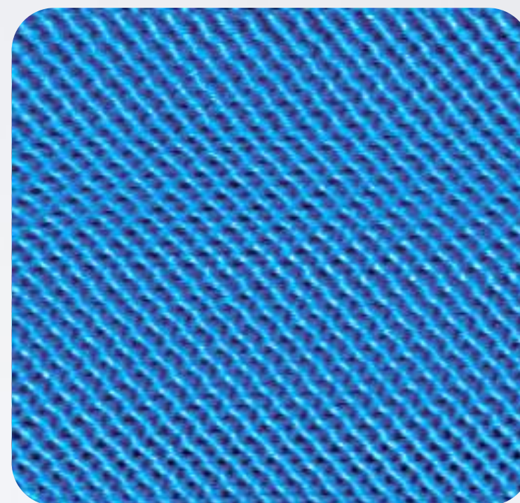
7×7 nm Calcite atomic resolution, AM-AFM in liquid
