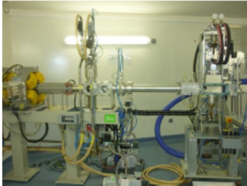
Beamline with irradiation station accomodating rabbits with samples
